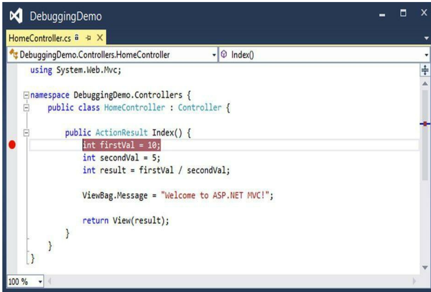
Figure 14-8 . Applying a breakpoint to the first statement in the Index action method
