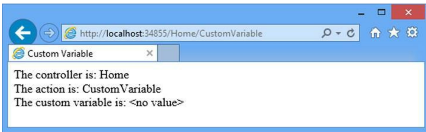
Figure 15-10. Detecting when a URL doesn't contain a value for an optional segment variable
