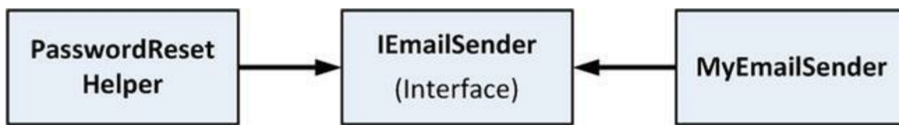
Figure 3-5 . Using interfaces to decouple components
